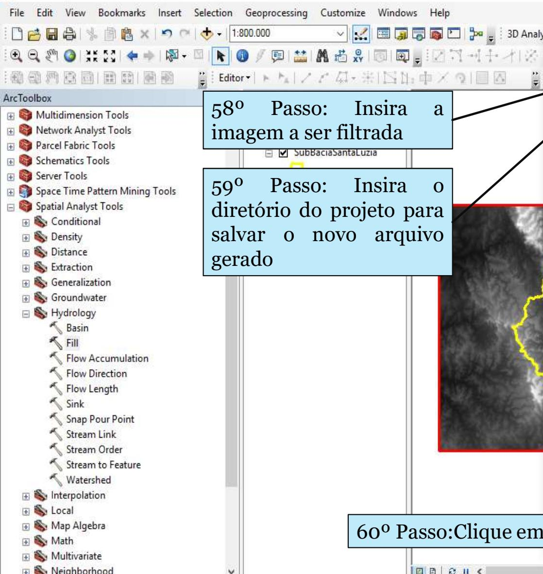
Geoprocessing tool that fills sinks in a surface raster to remove small imperfections in the data.
